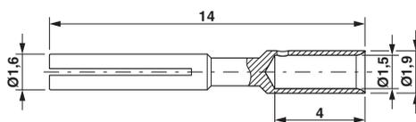
Crimpkontakt, Durchmesser: 1,0 mm
