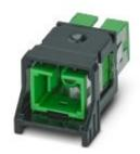
Fiber optic coupling, type: SC, degree of protection: IP20, material: PBT, connection method: Coupling, cable outlet: straight
