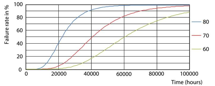
LEDtube MAS SLR 14W 60K FailureRate-LED
