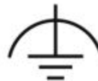
Connection of the protective equipotential bonding conductor
