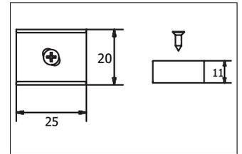
Halter-Set. Abmessung Profil: L: 25 mm x B: 20 mm x H: mm.
