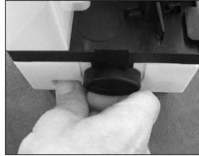
2. Clean the float switch and the condensate collector.
