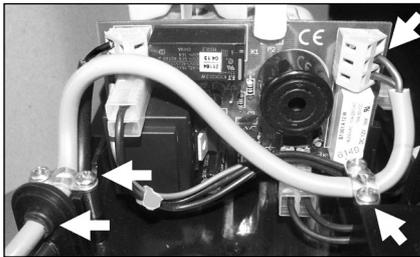
Insert the alarm connection cable into the condensate pump housing parallel to the mains cable. To do so, the second opening in the cable grommet must be opened up.
