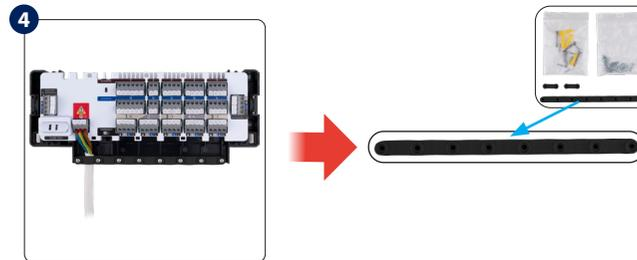
For safety use fastening strap to prevent power supply / thermostats wires from falling out.
