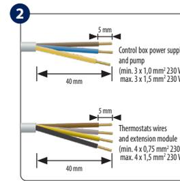
Remove the appropriate piece of insulation from the wires.
