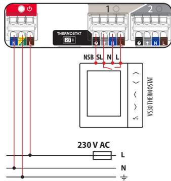
• Connecting a 230 V thermostat to the CB500X control box extension (e.g. SQ610)
