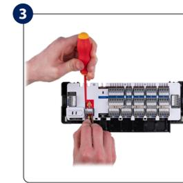
Connect the wires to the spring clamps according to the wiring diagrams. You can run the cables in the tunnel under control box housing.
