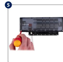
Make sure that all the wires are properly connected, mount top cover and power up the control box - the red power indicator LED will be illuminated.
